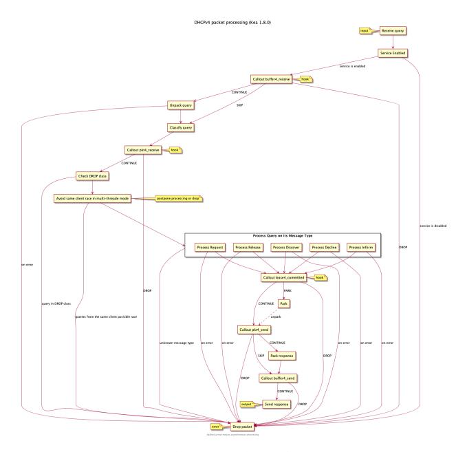
Fig. 2: DHCPv4 packet processing
